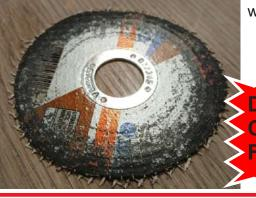
DO NOT USE A CUTTING DISK FOR GRINDING
